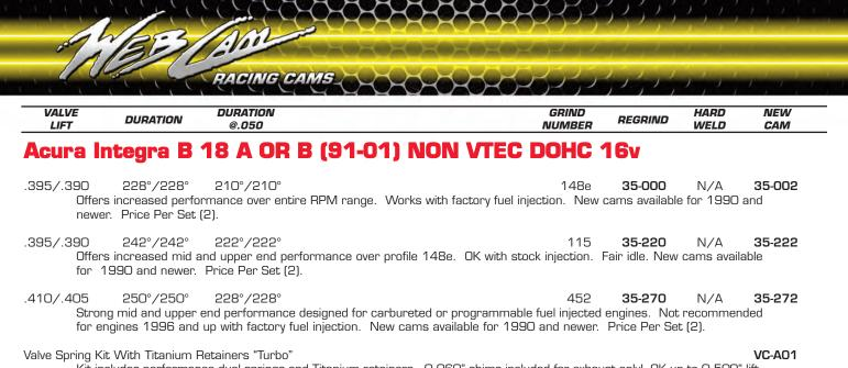
Kit includes performance dual springs and Titanium retainers. 0.060" shims included for exhaust only! OK up to 0.500" lift. Installed at 1.390" - 1.400". Fits B18A engine. Price Per Set (16).
